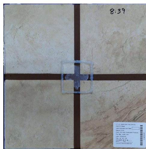
Figure 9 Mapei™ Ultracolor® Plus FA (Mahogany) grout sample at 28 days of curing, 24 hours after application of Deionized Water droplet
