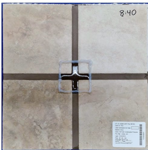
Figure 25 TEC® Power Grout® (Espresso) grout sample at 28 days of curing during efflorescence emittance test
