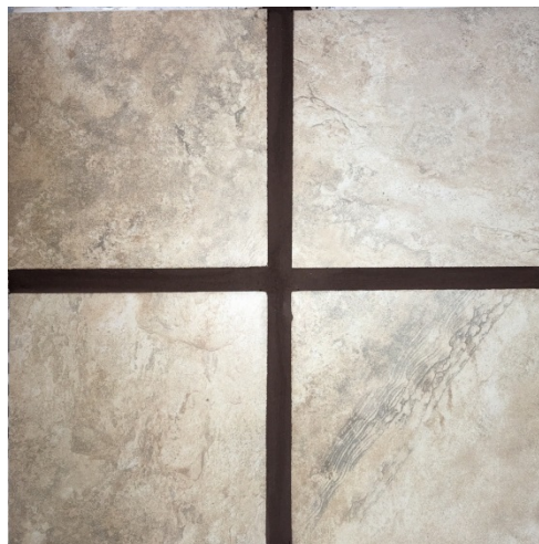
Figure 3. Mapei™ Ultracolor® Plus FA (Mahogany) grout sample before efflorescence emittance test
