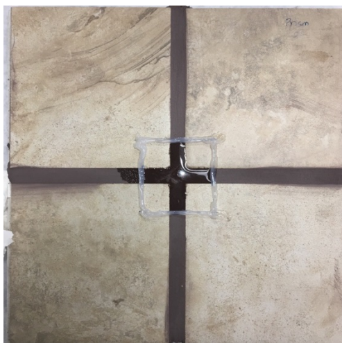
Figure 22 Prism® Color Consistent Grout (Sable Brown) grout sample at 28 days of curing during efflorescence emittance test
