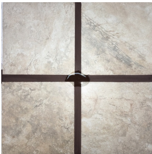
Figure 4 Mapei™ Ultracolor® Plus FA (Mahogany) grout sample at 3 days of curing during efflorescence emittance test
