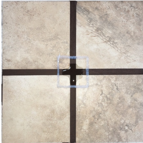
Figure 13 LATICRETE™ PERMACOLOR® Select (Espresso) grout sample at 7 days of curing during efflorescence emittance test
