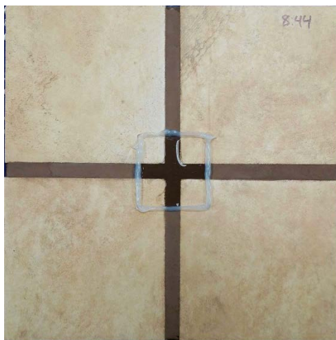
Figure 25 TEC® Power Grout® (Espresso) grout sample at 3 days of curing during efflorescence emittance test
