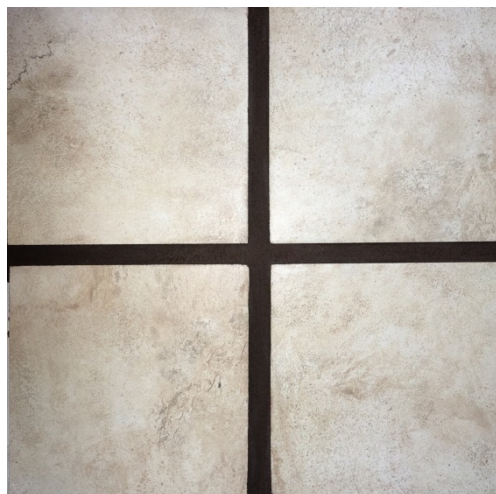
Figure 10 LATICRETE™ PERMACOLOR® Select (Espresso) grout sample before efflorescence emittance test
