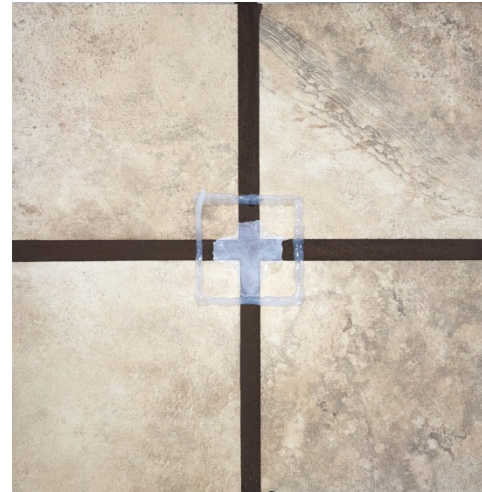
Figure 14 LATICRETE™ PERMACOLOR® Select (Espresso) grout sample at 7 days of curing, 24 hours after application of Deionized Water droplet
