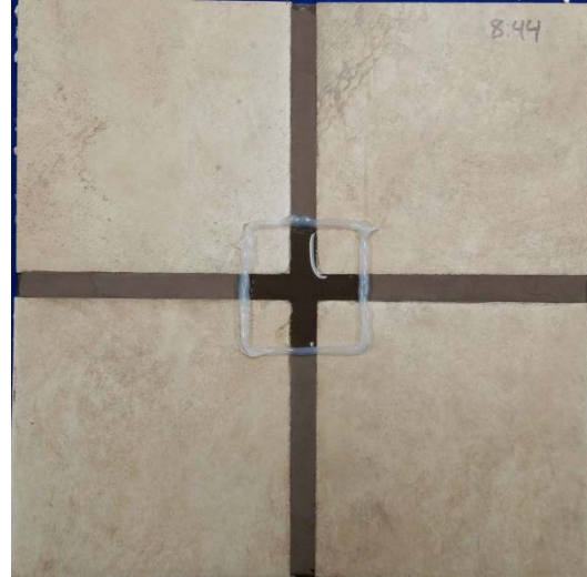
Figure 2 Grout sample specimen after 2 ml of deionized water have been applied in the center of grout lines
