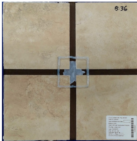
Figure 16 LATICRETE™ PERMACOLOR® Select (Espresso) grout sample at 28 days of curing, 24 hours after application of Deionized Water droplet
