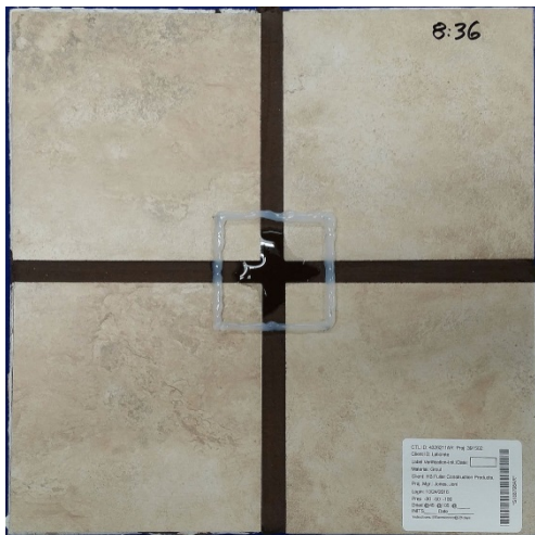
Figure 15 LATICRETE™ PERMACOLOR® Select (Espresso) grout sample at 28 days of curing during efflorescence emittance test
