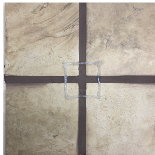
Figure 23 Prism® Color Consistent Grout (Sable Brown) grout sample at 28 days of curing, 24 hours after application of Deionized Water droplet
