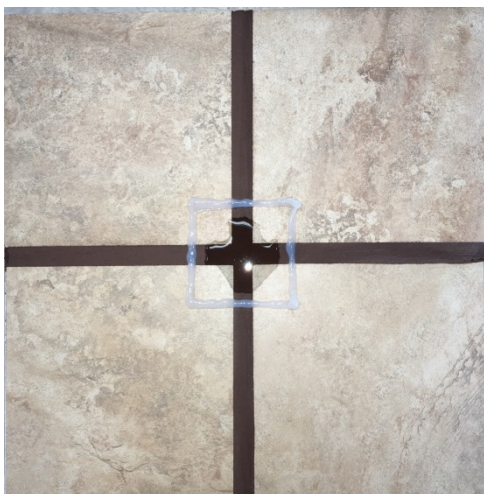
Figure 6 Mapei™ Ultracolor® Plus FA (Mahogany) grout sample at 7 days of curing during efflorescence emittance test
