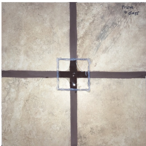
Figure 20 Prism® Color Consistent Grout (Sable Brown) grout sample at 7 days of curing during efflorescence emittance test
