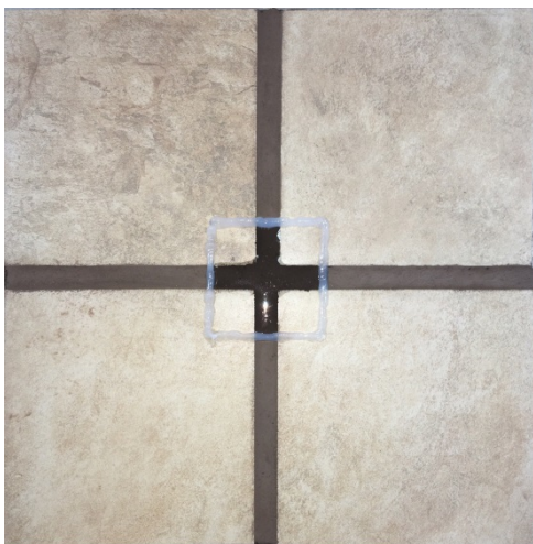
Figure 27 TEC® Power Grout® (Espresso) grout sample at 7 days of curing during efflorescence emittance test
