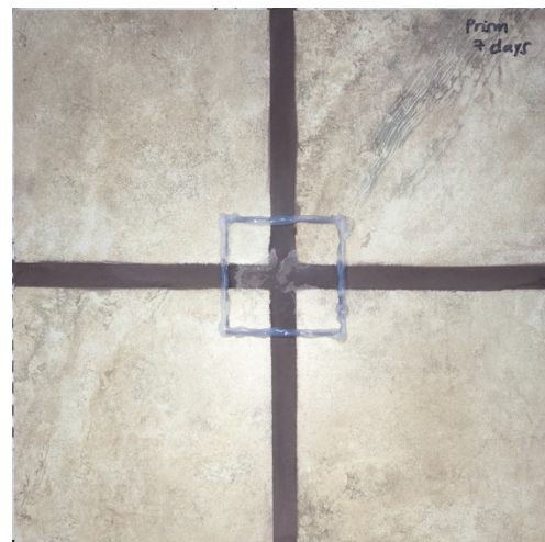
Figure 21 Prism® Color Consistent Grout (Sable Brown) grout sample at 7 days of curing, 24 hours after application of Deionized Water droplet
