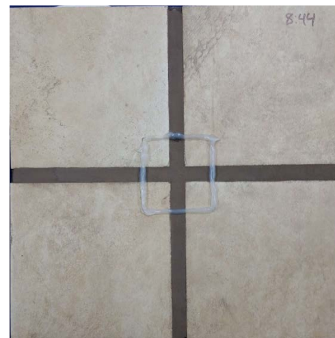
Figure 26 TEC® Power Grout® (Espresso) grout sample at 3 days of curing, 24 hours after application of Deionized Water droplet
