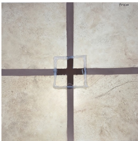
Figure 18 Prism® Color Consistent Grout (Sable Brown) grout sample at 3 days of curing during efflorescence emittance test
