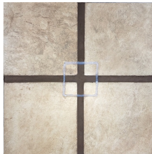
Figure 28 TEC® Power Grout® (Espresso) grout sample at 7 days of curing, 24 hours after application of Deionized Water droplet
