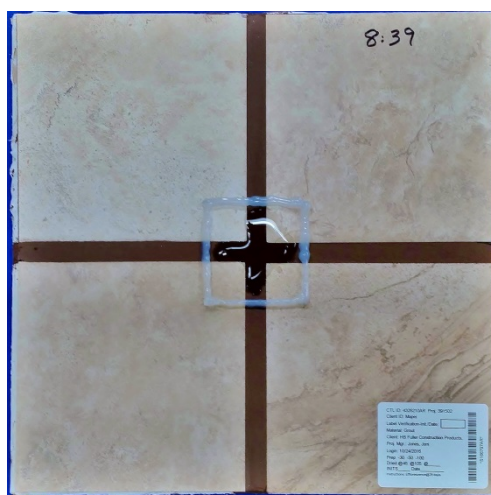
Figure 8 Mapei™ Ultracolor® Plus FA (Mahogany) grout sample at 28 days of curing during efflorescence emittance test
