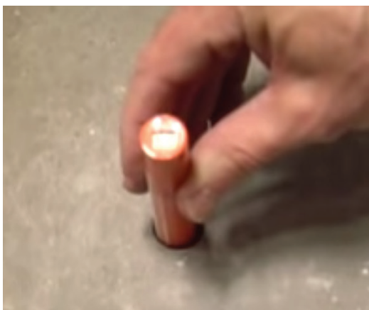
Test the substrate's moisture levels using the ASTM F-2170 test.
